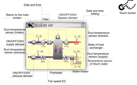
Remote control displays alarm symbol if a failure disturbs the work of the device. The sign, that indicates a specific problem will appear in information window.
