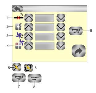
Next locked settings window has rotary heat exchanger settings. User in this window can enter period of rotor rotation also switching time and pulse rate per minute of rotary heat exchanger.
